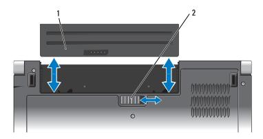
1 2 battery release latch battery
